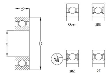
B = 13 Ball grade = 3 C (KN) = 13.8 C0 = 8.3 d = 30 D = 55 Max rpm. = 19000 Type = 6006
